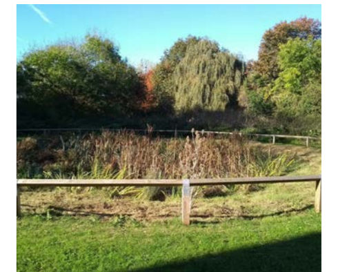
Fig. 77 - Drainage ponds should not be isolated and fenced features
