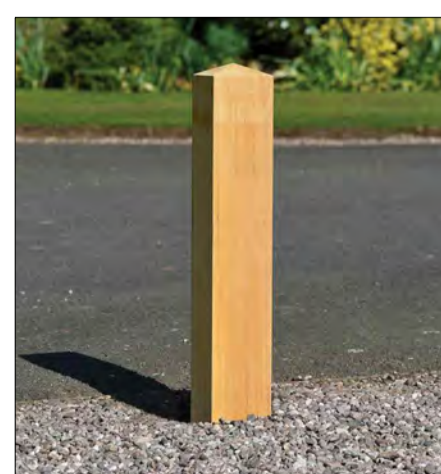
B01 Proposed Timber Bollard | Supplier: Broxap | Product Code: BX17 Painted - Square | Dimensions: 150x150mm x1000mm | Fixing: Fixed into concrete footing. Reflective bands in rebates. Granite setts surrounded.
