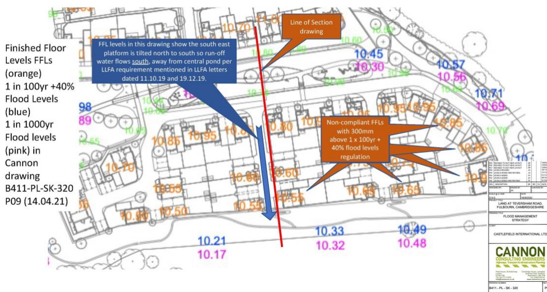
Figure C7. Site plan produced on 14.04.21 indicates that the north-eastern development platform slopes from north to south, in conflict with contemporaneous site section (figures C6 and C8).
