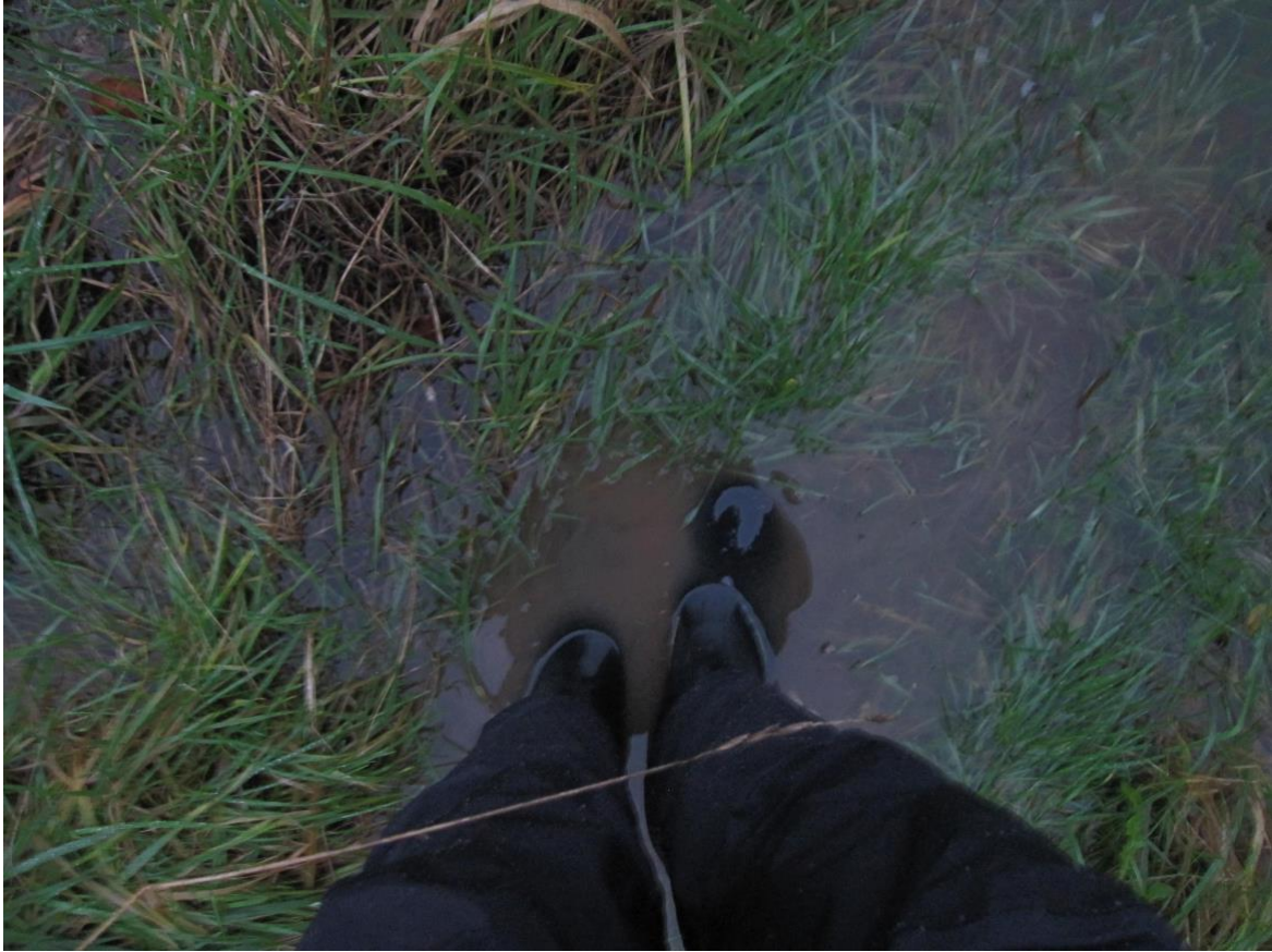
Figure A6. Standing water on many parts of the development site is a regular occurrence. Site of south-eastern development platform (date 23 November 2014). The waterlogging is in keeping with there being clay here, rather than it being free draining chalk.
