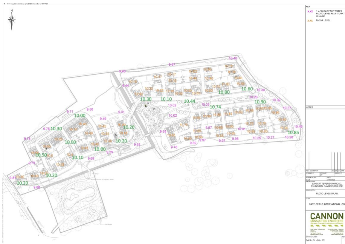
Figure E19. Finished floor levels are not 300mm above road levels, with some at or below road levels.
