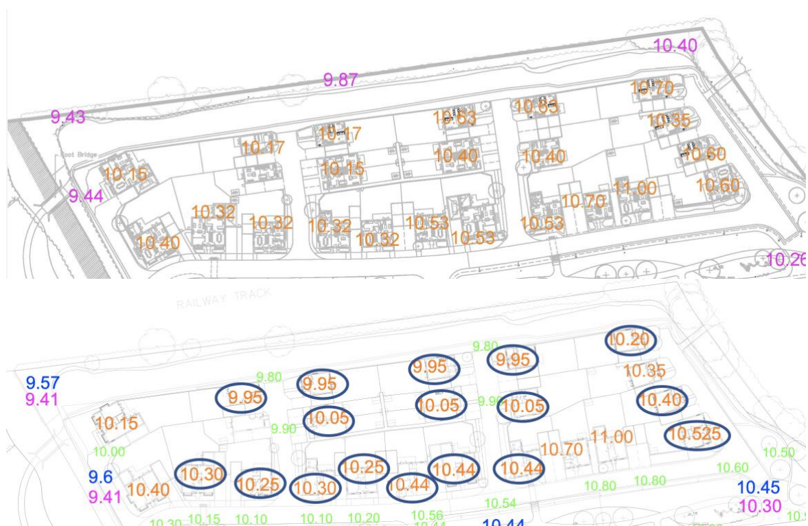
Figure E2. New flood management plans presented for the Appeal, shows very substantial changes in finished floor levels on the northern development platform compared with the previous version (P09) of the flood mitigation strategy that was rejected by the Planning Committee in October 2021.
