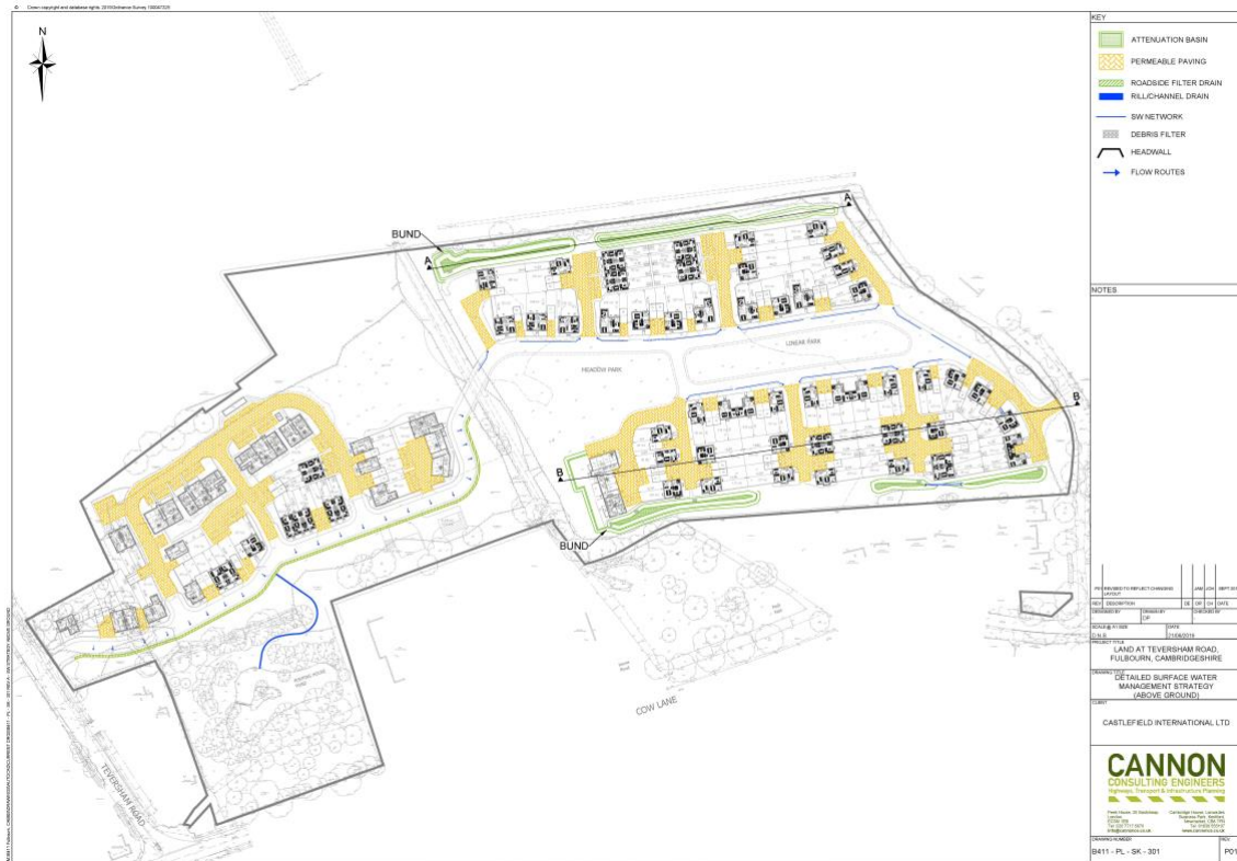
Figure C2. Original surface water and drainage plans (P01, September 2019), comprising crated storage and 5 bio-retention ponds.
