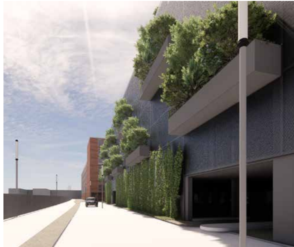
Expanded metal mesh with external planters
