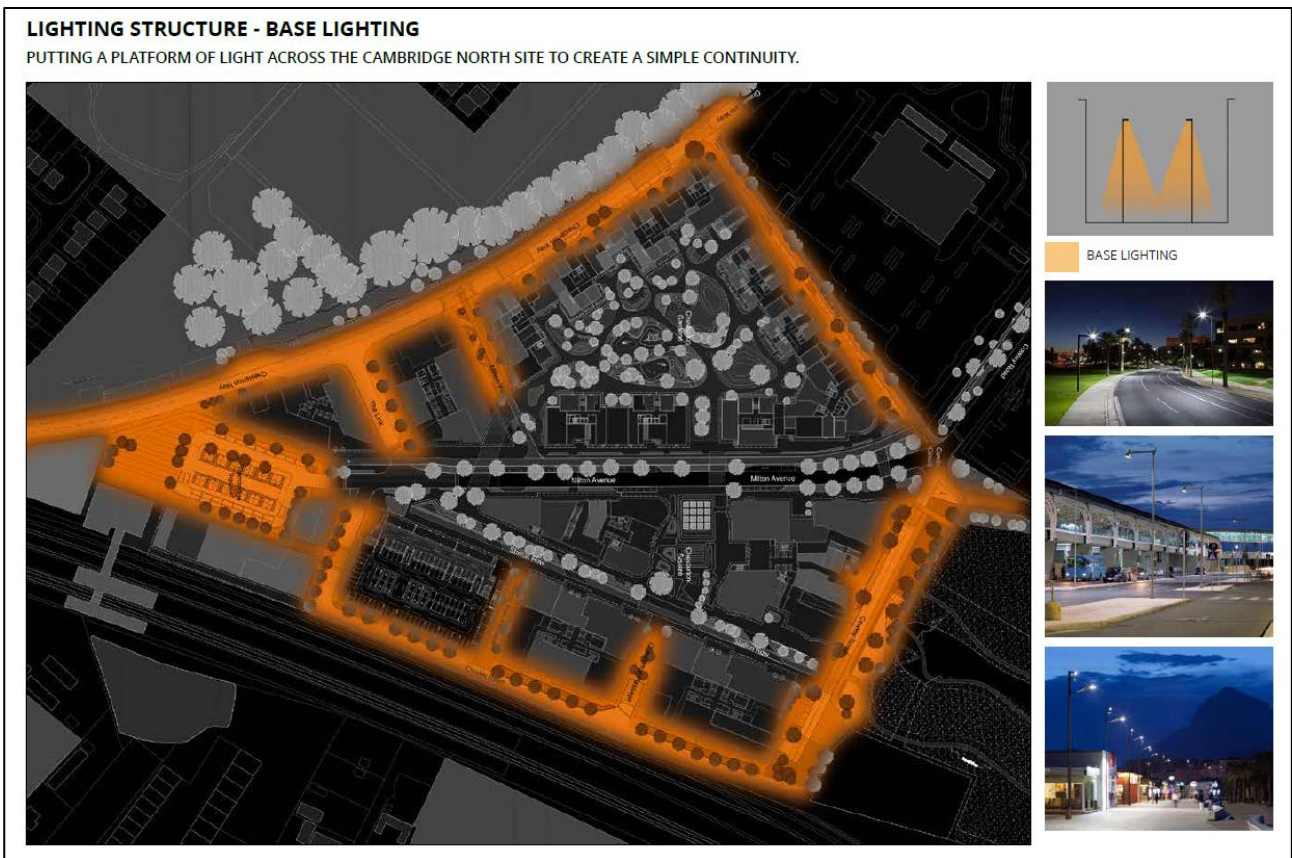
Figure 23 - Base lighting, it is noted as this element continues the existing lighting systems ensuring compliance with E2 at the site boundary, as measured in the baseline assessment.
