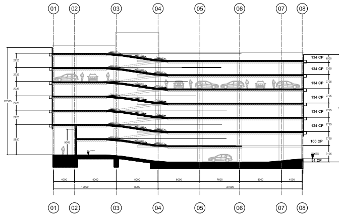
01.12.2021 - 6 Storeys increased floor to floor height
