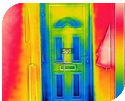
A thermal imaging camera spots where heat is escaping
